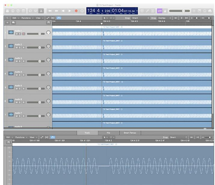
*A T2 audio glitch captured during recording. The entire waveform should be smooth and uninterrupted. Some glitches like this could probably be edited, but errors like these can destroy a recording.*
