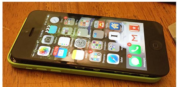
Your Home button won't work at this point, because when you press it on the front half of the iPhone, it pushes contacts onto two gold pins on the back half. If you want to make sure that the Home button is connected upstream, you can bridge these two gold pins with a screwdriver — the iPhone should act as if you pressed the Home button.
