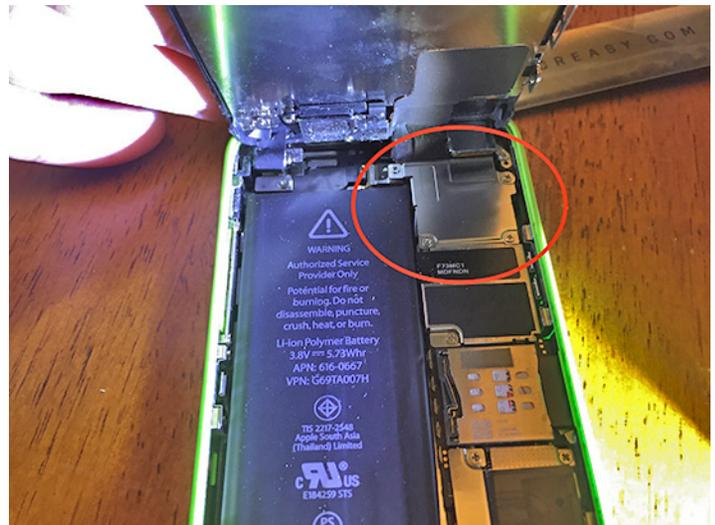
Begin removing the screws from the shield, but be aware that the screws are all different lengths, so you need to
